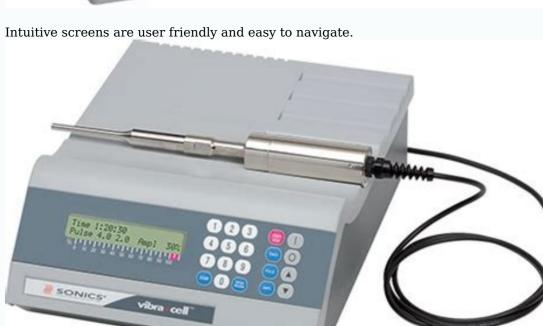
The 750 watt power supply has the capability of operating our largest assortment of horns and accessories. A standard 1/2" diameter probe (50 - 250mL volumes) with replaceable tip is included with the system. Part No. VCX 750A can be used to order the system without the standard probe. The VCX 500 offers 500 watts of power to handle a range of liquid processing applications.
